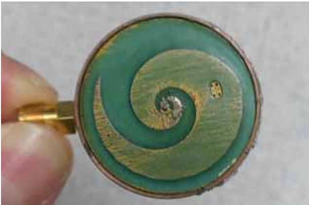
Figure 3 2.5 cm diameter tapered log spiral microstrip antenna encapsulated together with the radiometer electronics printed circuit on the back surface of antenna inside a cylindrical copper tube with 1 mm wall thickness.
