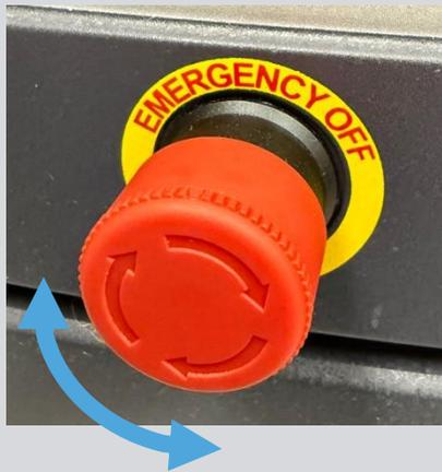
Button can be reset by twisting with a slight press until it returns to its default state
