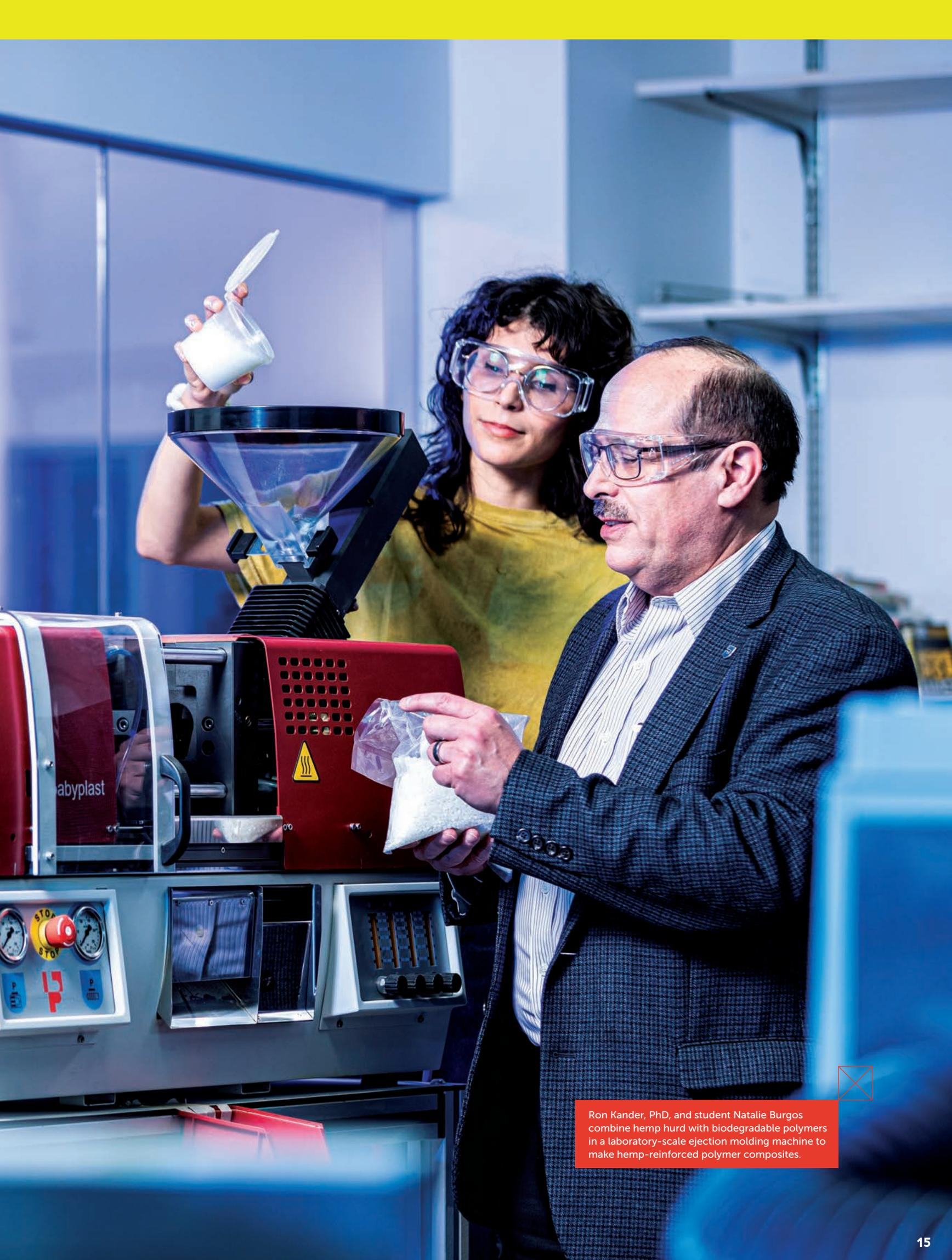
Ron Kander, PhD, and student Natalie Burgos combine hemp hurd with biodegradable polymers in a laboratory-scale ejection molding machine to make hemp-reinforced polymer composites.
