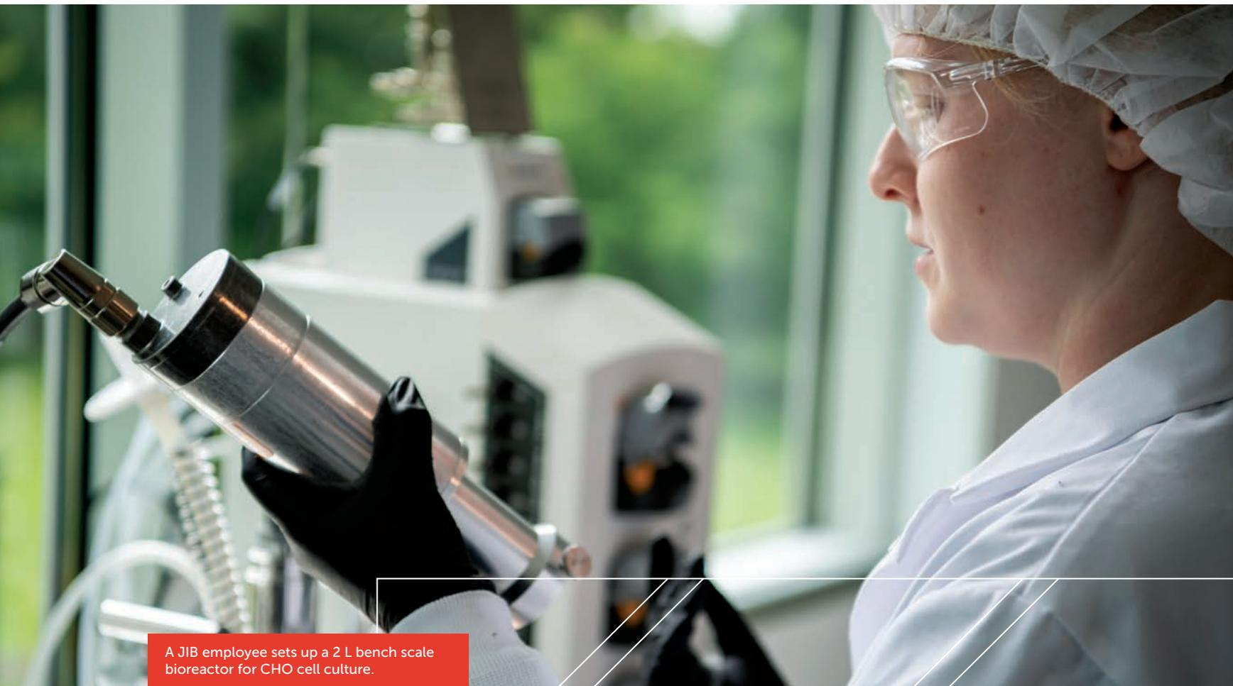
A JIB employee sets up a 2 L bench scale bioreactor for CHO cell culture.
